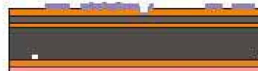
Poly-silicon (2 $\mu$ m) **actuators** are deposited and structured
